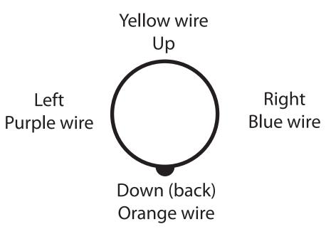
Joystick Highhat wiring diagram
